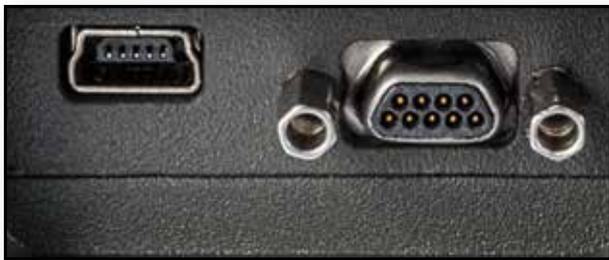
The USB connection is used for charging the battery or for transmitting data to a personal computer. The RS-232 cable is used for connection to the FMM Digital Tester. The DFC also has Bluetooth®.
