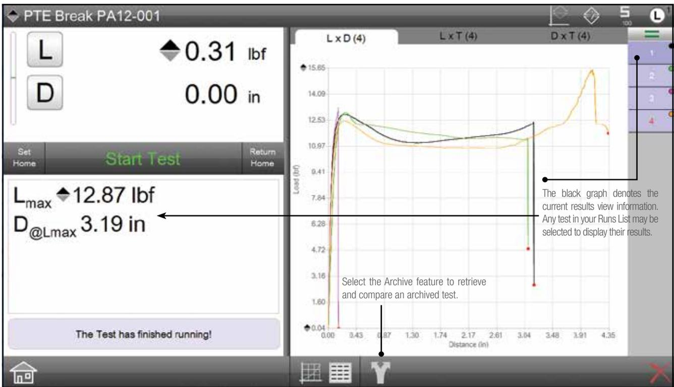
Compare the graphical results of multiple tests that you select. Individual graphs are color-coded and referenced to the test in the Runs List. You can also retrieve archived tests for making a graphical comparison. For example, you can compare a "benchmark" result from a year ago to a current result.
