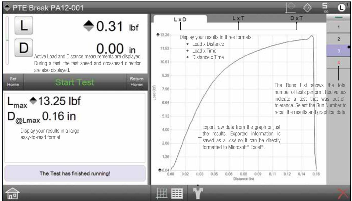
When the test concludes, your L1 software shows your results in numerical and graphical formats. Essential measurements are displayed in easy-to-interpret formats. You can Start and Stop a test using the touchscreen display; manually set the home position and return the crosshead to home position, and zero your load (L) and distance (D) measurements.
