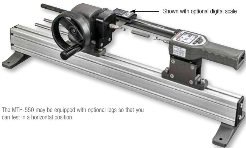
The MTH-550 may be equipped with optional legs so that you can test in a horizontal position.
