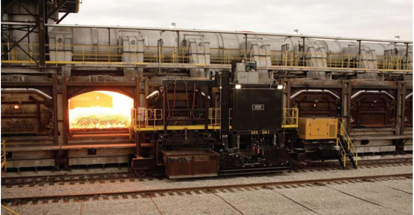
Fig. 20 Coke transfer car equipped with AP bearings
