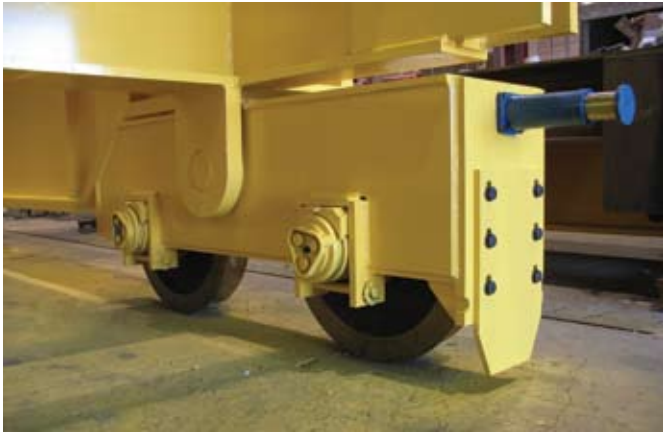
Fig. 5 Standard end cap design
