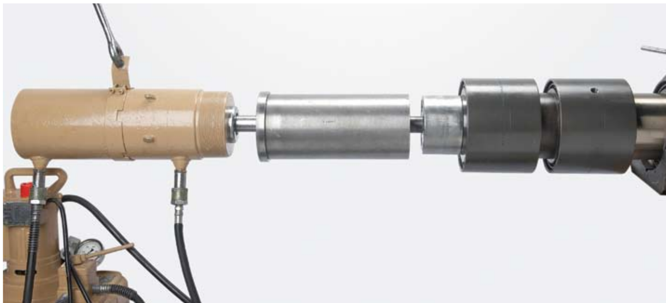
Fig. 28 Tooling used to push bearing onto shaft
