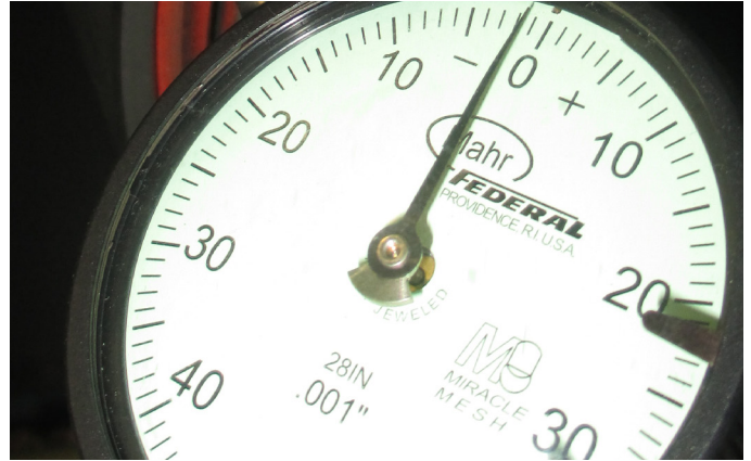
Fig. 12. The bearing lateral endplay should be 0.001 in. to 0.015 in. (Amtrak 0.001 in. to 0.020 in.).
