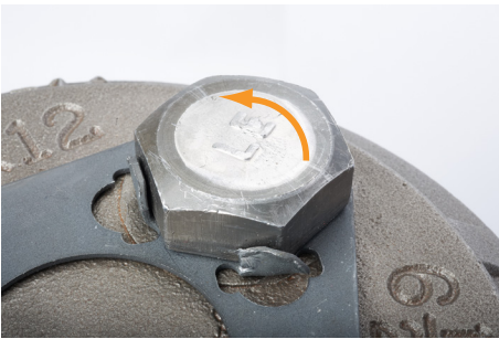
Fig. 9. Shows INCORRECT position. This position will not resist loosening (the arrow indicates loosening direction of the cap screw).
