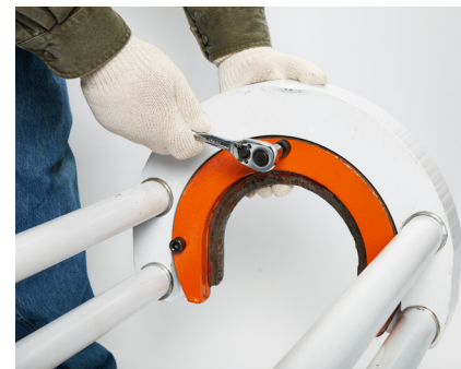
Fig. 15. Ensure the pulling shoe adapter is securely seated inside the pulling shoe.
