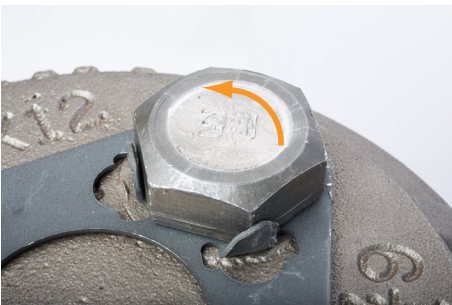
Fig. 10. Correct position of tab against cap screw head flat. This position helps resist loosening of the cap screw (the arrow indicates loosening direction of the cap screw.).
