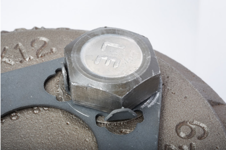
Fig. 8. If cap screw head is centered on a locking plate tab, see figures 9 and 10 below.
