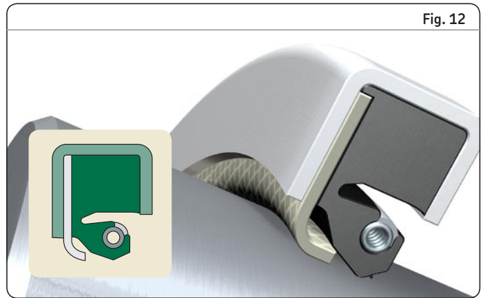
HDSG2 with lip position and direction to provide improved lubricant retention
