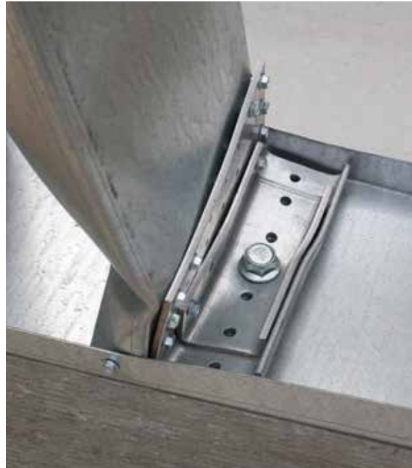
RCKW Assembly Test with Member Failure
