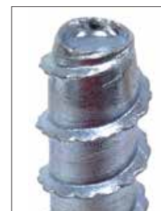
Serrated teeth on the tip of the Titen HD screw anchor facilitate cutting and reduce installation torque.
