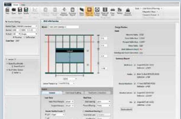
Design automation tools for framed wall openings, x-braced and sheathed shearwalls, floor joists, rafters and stacked walls
