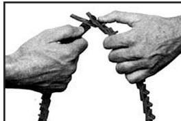
3. Rotate belt end with tab 90°.
