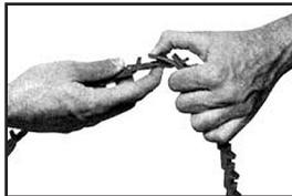
3. Flex belt further and insert second tab through end link by twisting tab with thumb.
