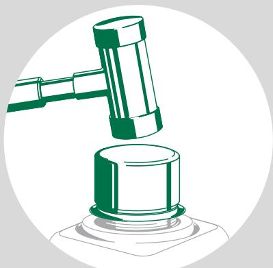
Tap installation tool with mallet until sleeve is seated on shaft over the marked area. Remove installation tool.
