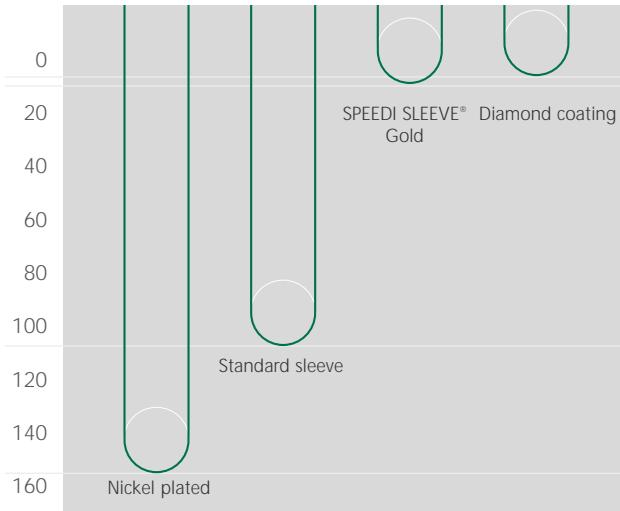
Testing in highly abrasive conditions demonstrates how the hardened surface of SPEEDI-SLEEVE® GOLD resists wear
