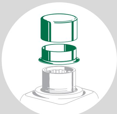
Place SPEEDI SLEEVE® on to the shaft and then place special installation tool over the sleeve.
