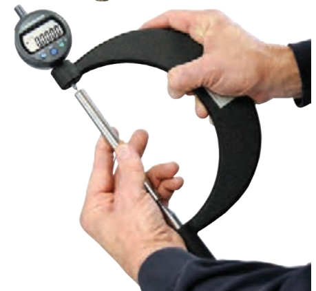
Setting PD-8001-RSC with Rod Standard
