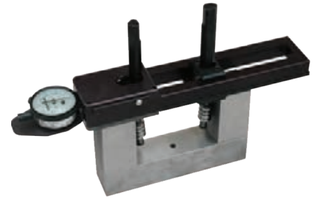
Setting an MRP-5001 with Frame Style Standards
