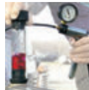
NO LEAK PRESENT (NO CHANGE IN FLUID COLOR)
