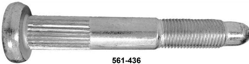
561-436 M14 x 1.5 x 104mm Knurl diameter: 16mm
