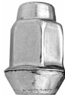
559-190 M12R x 1.5 19mm Hex 36mm Height Dometop Capped Stainless Steel
