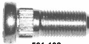
561-102 M12 X 1.25 x 32mm Knurl diameter: 12.9mm (Code: D.2.0)
