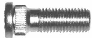
561-140 M12 x 1.5 x 37mm Knurl diameter: 14.4mm (Code M.1.8)
