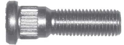
561-312 M12 x 1.5 x 44.4mm Knurl diameter: 14.17mm
