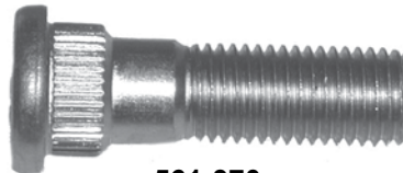
561-370 M12 x 1.5 x 44mm Knurl diameter: 15.8mm
