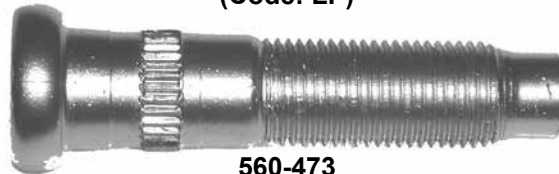
560-473 9/16-18R x 2-5/8" Knurl diameter: .622 (Code: CX)
