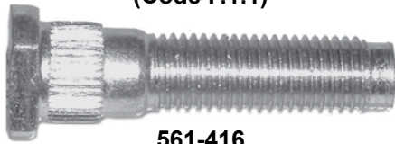
561-416 M12 x 1.5 x 52mm Knurl diameter: 14.8mm
