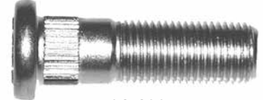
561-100 M12 x 1.25 x 39mm Knurl diameter: .12.9mm (Code: D.1.0)
