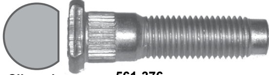
561-376 M12 x 1.5 x 49mm Knurl diameter: 13.9mm
