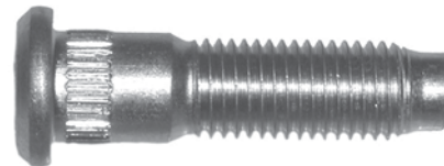
561-249 M12 x 1.5 x 46mm Knurl diameter: 15.37mm
