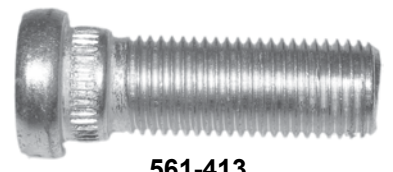
561-413 M14 x 1.5 x 43mm Knurl diameter: 15.7mm (Code PU)
