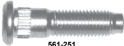
561-251 M12 x 1.5 x 51mm Knurl diameter: 13.5mm (Code F.1.1)
