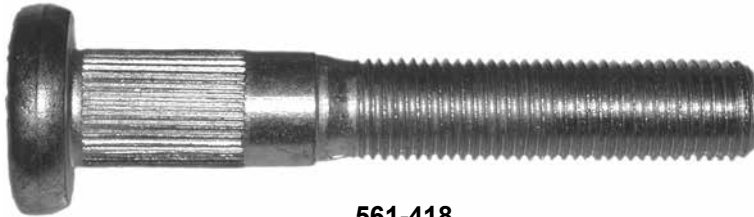
561-418 M14 x 1.5 x 91mm Knurl diameter: 15.7mm (Code DL)
