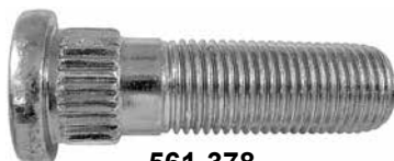
561-378 M12 x 1.25 x 42mm Knurl diameter: 14.35mm
