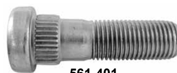
561-401 M12 X 1.25 x 42mm Knurl diameter: 14.43mm
