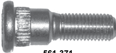
561-371 M12 x 1.5 x 43.8mm Knurl diameter: 17mm
