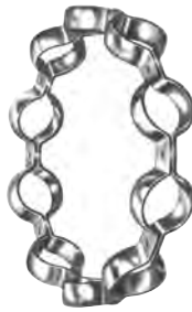
Fig. A-2. Pressed-steel welded cage.
