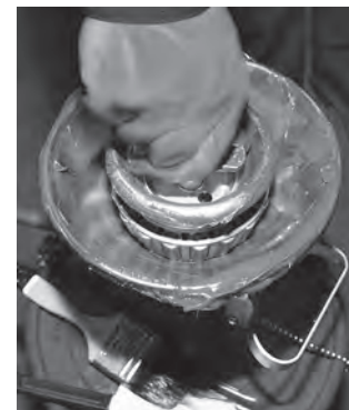
Fig. D-11. Mechanical grease packer.
