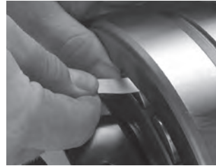
Fig. D-3. Measure RIC before installation.
