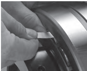
Fig. D-7. Measure RIC before installation.
