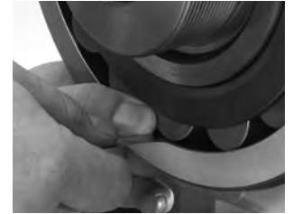
Fig. 4. During mounting, the RIC should be checked at the unloaded roller.
