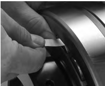
Fig. 7. Measure RIC before installation.
