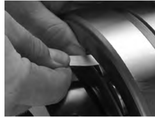
Fig. 3. Measure RIC before installation.
