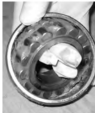
Fig. 10. Grease can easily be packed by hand.
