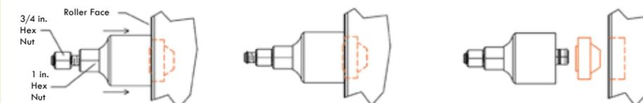
1. Push conveyor-roller puller into bearing and up to roller face.
