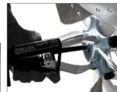
Makes cooling fan removal a one-man operation.
