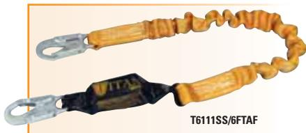
**Titan Stretch Pack-Type Shock-Absorbing Lanyards** contract from 6-ft. (1.8 m) to 4-ft. (1.2 m) to reduce tripping hazard and smoothly expand to reduce fall forces while a back-up safety strap deploys for added fall protection.
