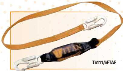
**Titan Pack-Type Shock-Absorbing Lanyards** include the shock absorber pack as an integral part of a standard lanyard. In the event of a fall, the pack smoothly expands to reduce fall forces while a back-up safety strap deploys for added fall protection.
