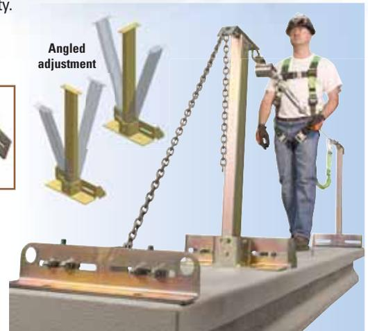
Complete system includes stanchions, tie-back brackets, chain connectors, slider brackets, energy absorber(s), line tension indicator, turnbuckle, cable and hardware. Attach to rebar, coil inserts or concrete expansion bolts.
