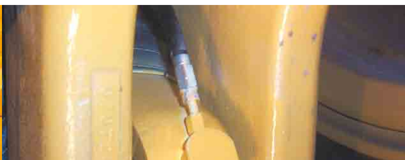
Inlet adaptor designed to protect the compression fitting
