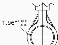
Copper Plated Acme Screw / Ductile Iron Body
