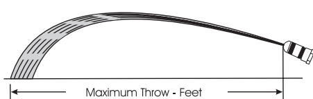
TIP SETTING "B" STRAIGHT STREAM SPRAY PATTERN
