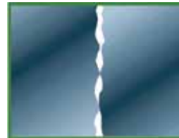
Typical press fit has 30% metal-to-metal contact.
