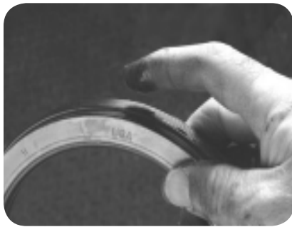
Lightly lubricate the O.D. and I.D. with the fluid being retained.
