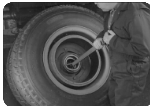
The SKF tool makes seal removal easy even on the largest heavy duty wheels.
