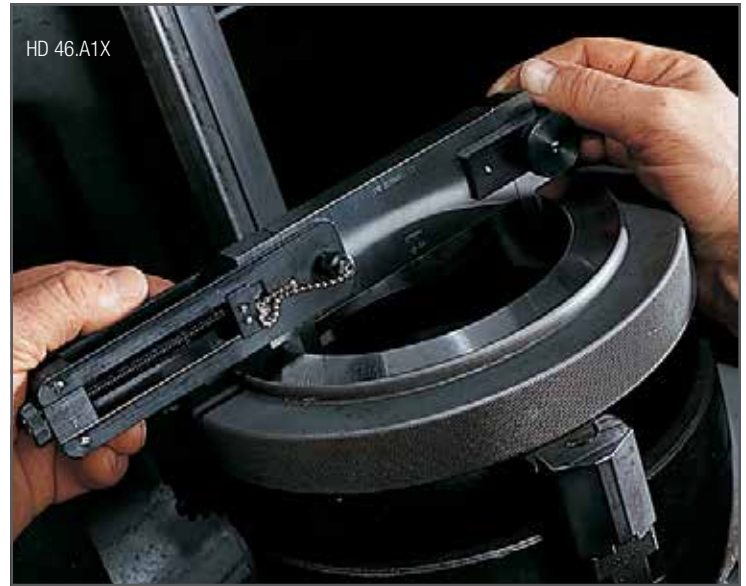
Snap gage is used to check inside dimensions of ring gage still mounted in internal grinder
