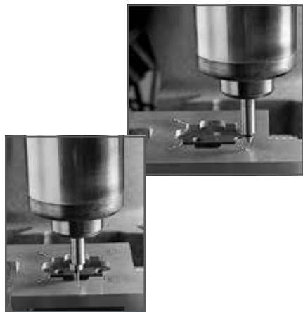
Above: Locating the center with 827MB Left: Locating the edge of a part with 827MA
